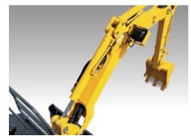
The boom cylinder is now mounted on top of the boom. This helps to avoid hitting it against obstacles when loading truck or digging deep. This design also increases the boom's pressing force, enhancing penetration into the ground.
